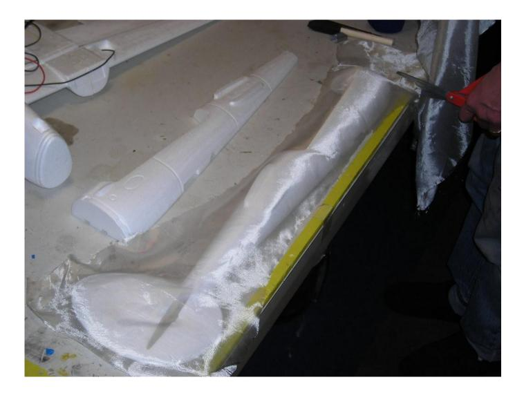
Apply the WBPU directly to the surface of the cloth, you do not need wet the foam surface first.
