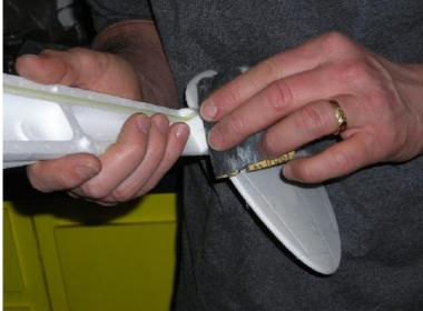
After edges are cleaned up, sand surfaces with 600grit sandpaper and apply second coat of WBPU. You can sand and apply 3<sup>rd</sup> coat if you like. I would not recommend using more than 3 coats for WBPU.
