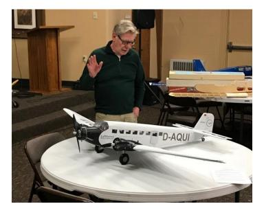
Joe Neidermayr had a nice looking Junkers 52 built from a kit. It was powered by three 3536 electric motors , had a 74-inch wingspan and weighed 9 pounds. Joe said the corrugated siding was homemade.
