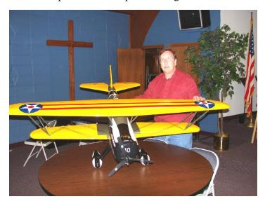
Steve Meyer had a very nice Great Planes ARF of a Curtiss P6E. This bipe was done in Army trainer colors of black fuse with yellow wings, covered with Monokote. The plane was powered with a Saito 180 4-stroke engine and had a 76-inch wingspan, making it IMAA legal. It weighed 14 pounds and had not flown yet.
