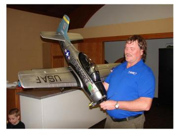
Gerry Dunne had a nice looking foam T-28 ARF done in silver with black trim. The detail on the place was very nice. It had a 55-inch wingspan and weighed in at 84 ounces. The manufacturer was JR and it was powered with a 4850 500 KV 700 watt motor. The battery was a 4-cell lipo. Gerry said it flew like a 'big trainer.
