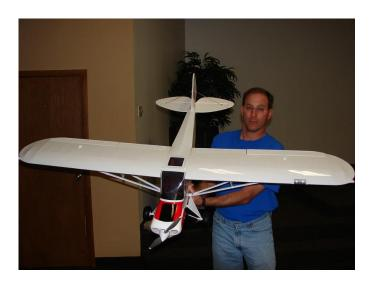
Tim Len had a Super J3 Cub PA-18 ARF done by E-Flite. This nice looking plane was powered by an E-Flite Power 46 and done in white with red and black trim. It had a 68-inch wingspan and weighed 6 pounds 10 ounces. He was swinging a 13x10 prop, had a 60 amp ESC in it and was powered by a 4-cell lipo. As of the meeting he had yet to do the maiden flight but was hoping to get it in sometime in the near future.
