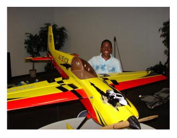
Newest TCRC member Dan Collier had a giant-scale 3D Slick 540 ARF. This plane was done in yellow and red with graphics Dan designed himself. He said it took him one week to assemble the 540 which was powered with an electric Hacker 80-10, which is equivalent to an 80 cc gas engine. The wingspan was 80 + inches and it weighed in at 23 pounds. Dan has 11 flights on the plane and says it has great flying characteristics.
