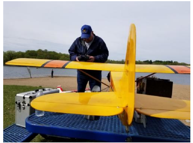
Checking out the control surface throws before a flight at Bush Lake.
