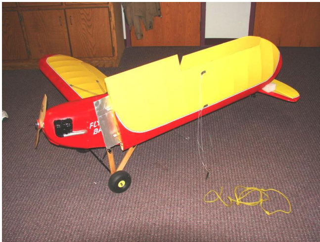
Stan Erickson's Fly Baby with the port wing folded back. (Photos by Jim Cook) ☺
