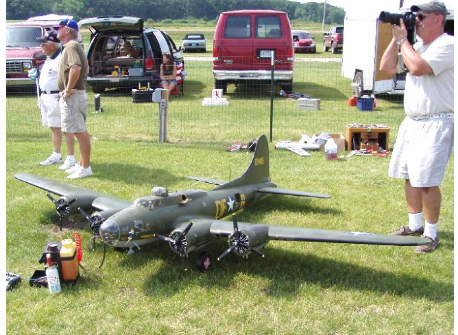
Cal Brandt's B-17 was powered by 4 OS 91 four-stroke engines.
