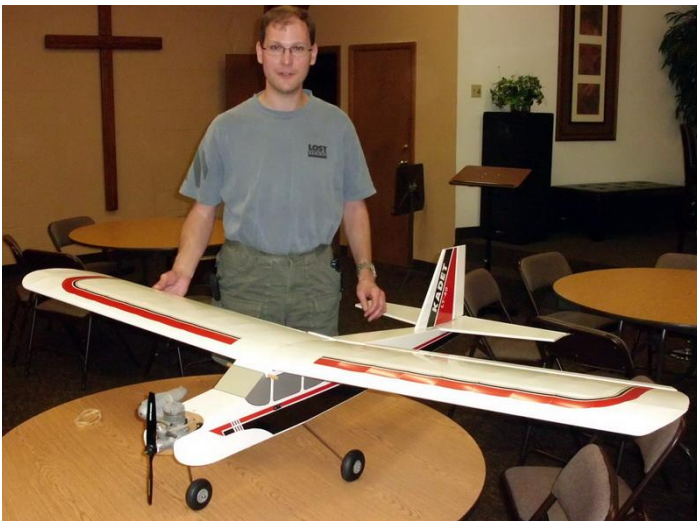
A nice looking Sig Kadet trainer with a 40-size two stroke engine ready to take its builder into the skies.
