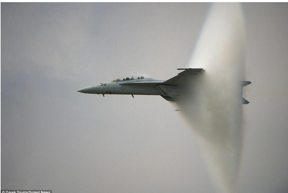
A Super Hornet fighter created the vapor cone as it approached the sound barrier at 760 mph. (Photo from Darek Slusta Solent News)
