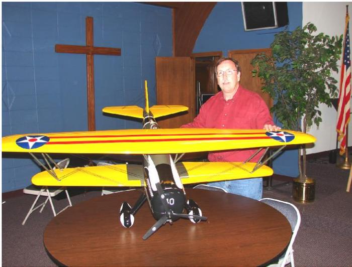
Steve Meyer had a very nice Great Planes ARF of a Curtiss P6E. This biplane was done in Army trainer colors of black fuselage with yellow wings, covered with Monokote. The plane was powered with a Saito 180 4-stroke engine and had a 76-inch wingspan, making it IMAA legal. It weighed 14 pounds and had not flown yet.
