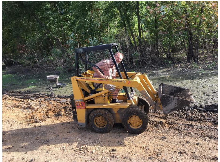
Jim Ronhovde's Mustang 310 skidsteer may have been small but it did a great job removing silt. (Photo by Jim Cook)
