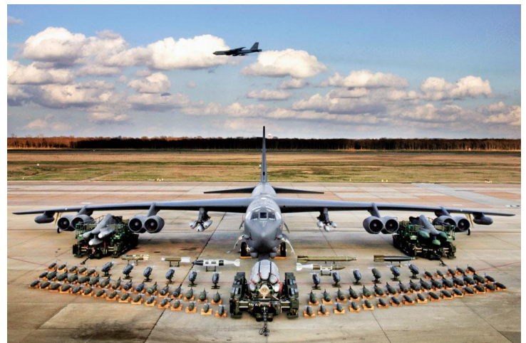
The B-52 can carry up to 70,000 pounds of ordnance, or the equivalent of 30 fully-loaded Cessna 172s.
