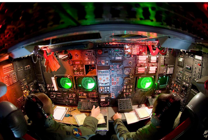
The navigator and radar navigator sit in the lower deck of the aircraft. These are the two seats that eject downward.
