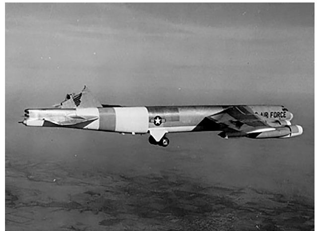
In 1964, a B-52 configured as a testbed to investigate structural failures flew through severe turbulence, shearing off its vertical stabilizer. The aircraft was able to continue flying, and landed safely.
