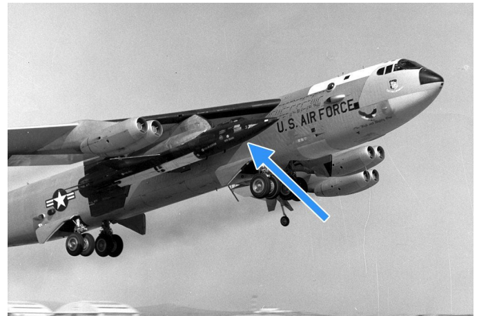
A B-52A was used to carry the North American X-15. The X-15 achieved the record for fastest manned powered aircraft, with a speed of Mach 6.72.
