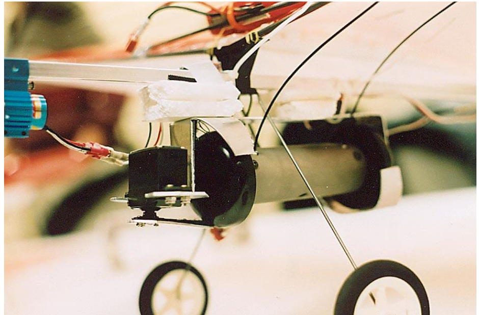
One of the U of M Center for Distributed Robotics robots in position under a Slow Stik prior to being dropped. (Photo by Jay Bickford)
